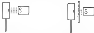
Fig.166 shows the standard set up for a Hall effect sensor. A moving magnet or a number of magnets in succession can be brought close to the sensor or a fixed magnet can be interrupted by a steel or iron vane. The vane can be in the form of sectors cut from a disc.
